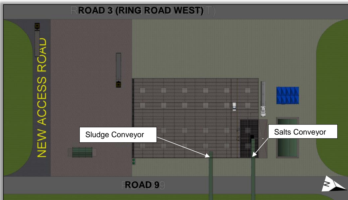
Figure 6: Position of Sludge and Salts conveyor at waste handling and storage facility
